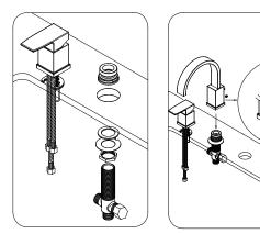
Unscrew the Allen screw in back of the spout. Pull apart the spout from its connector (do not unscrew). Separate the spout flange from the spout. Place o-ring underneath the spout flange and place the flange over the center hole between the handle and hand shower.
